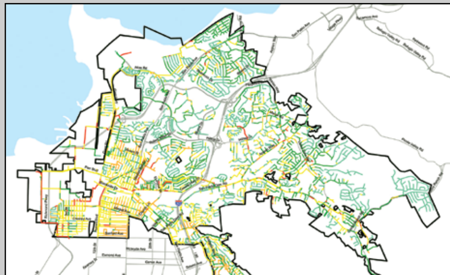
Figure 1. Collection system and WPCP rehabilitation projects were prioritized based on risk scores.
