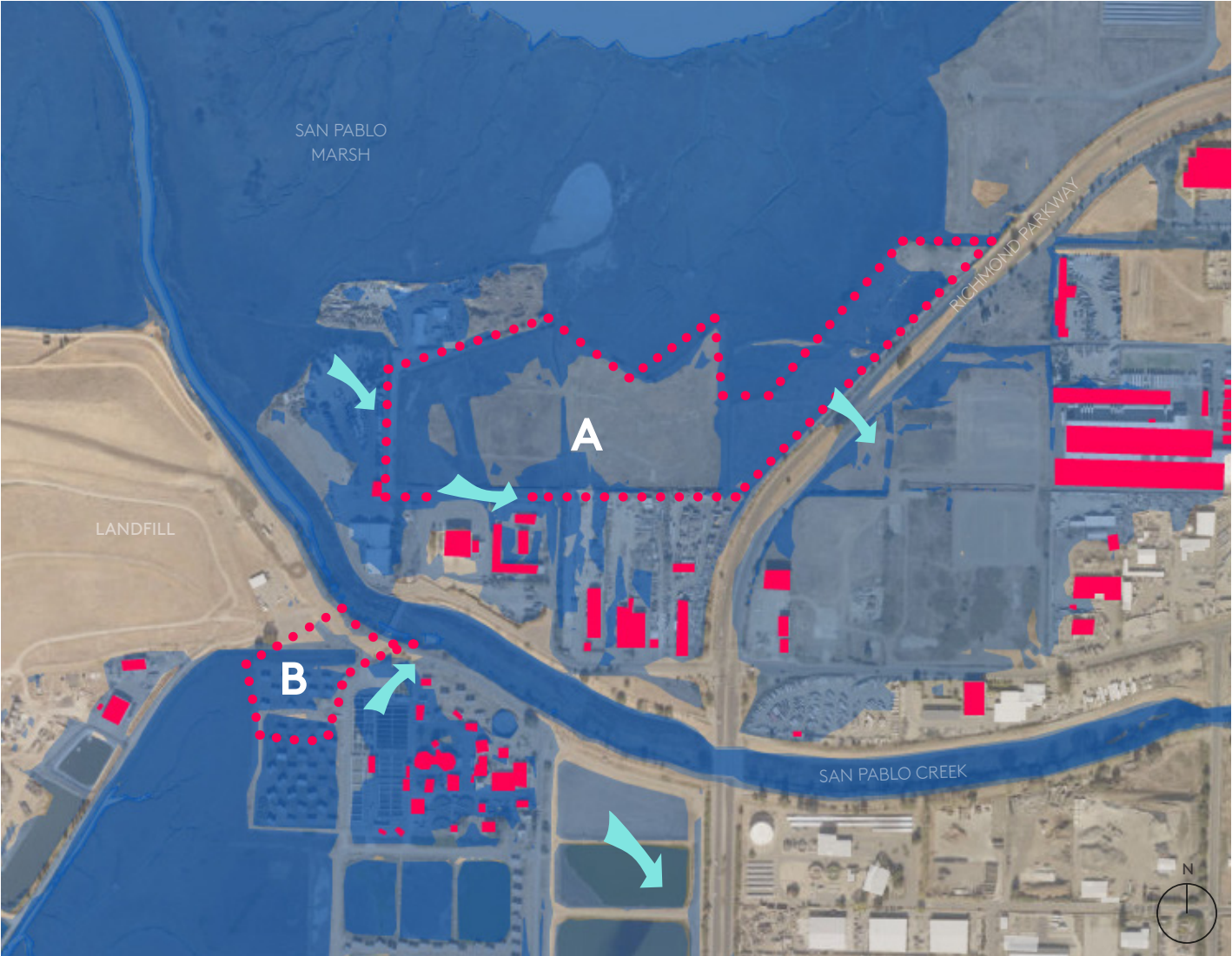
APPARENT FLOODING PATHWAYS (in light blue) in one enlarged portion of the North Richmond study area, based on lidar analysis.
